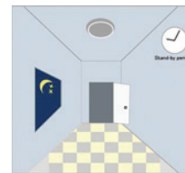
AT THE END OF THE WAITING TIME, NO MOTION IS DETECTED AND THE LIGHTS ARE TURNED OFF (OR KEPT ON AT THE WAITING BRIGHTNESS) IN THE THIRD STAGE.
