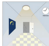
WHEN THE HOLDING TIME ENDS AND NO MOTION IS DETECTED, THE LIGHT BRIGHTNESS IS AUTOMATICALLY DIMMED AND THE WAITING TIME STARTS.
